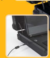
Power pack can also be operated with **external power pack** without batteries
